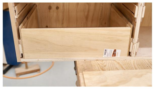
The width of this front panel will be the exact width of the rest of the parts. You'll want to make it so that it not tight – there should be some play for the drawer to slide freely.
