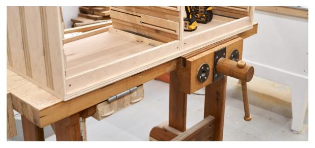
Then the middle stretchers were glue in and the back panel screwed on, and here's what it looks like fully assembled:
