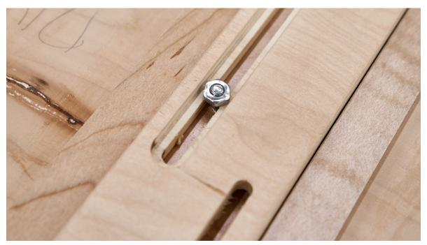
I used super glue to lock the nut in place and keep it from unscrewing.
