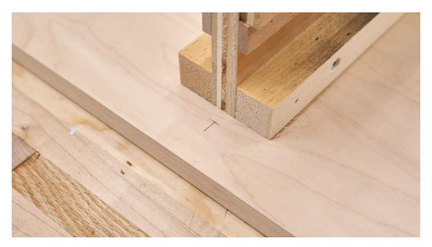
This gets it close, but then you need to fine turn it making the distance on both side of the divider panel as equal as possible. It's very important for the drawers to take the time to make sure these panels are both parallel and spaced accurately. Ideally, you want all of the drawers to be exactly the same width to save time when cutting out the parts – there are a lot of parts!
