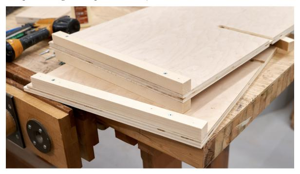
Important to put the cleats on the right side of the side panels – it's on the inside where the rabbet is. The divider gets a cleat on both sides.
