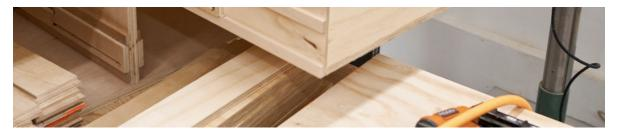
This one was a little tight fitting, so I planed a bit off the drawer runners to improve the fit:
