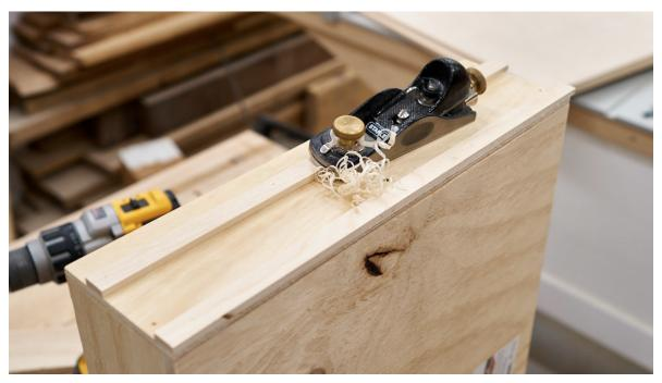
The upside of making the slides from wood is that they are very easy to adjust. Just need to be mindful of the pins driven in to hold the runners on, but those are typically driven below the surface. Sanding also works, though.
