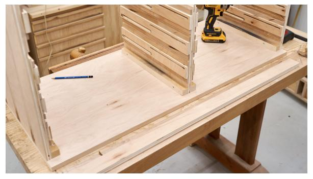
Then fasten it in place with 1-1/2" wood screws through the cleats and into the underside of the top panel.
