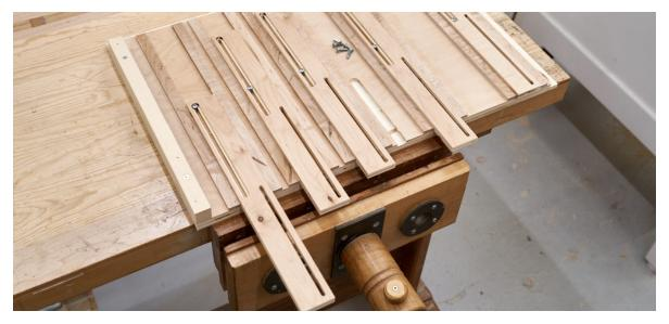
You snug the screw down, then back it off two turns. The head needs to be below the surface, so check that and make the slots deeper if needed.
