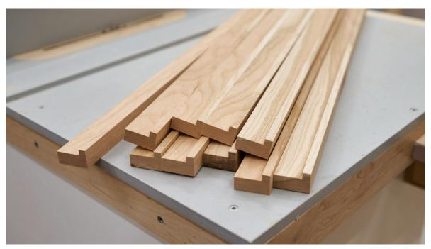
The piece I used had a lot of sapwood and I was able to hide most of that when cutting out the pulls. These get fastened to the top of the plywood fronts with glue and 1-1/4" brads.
